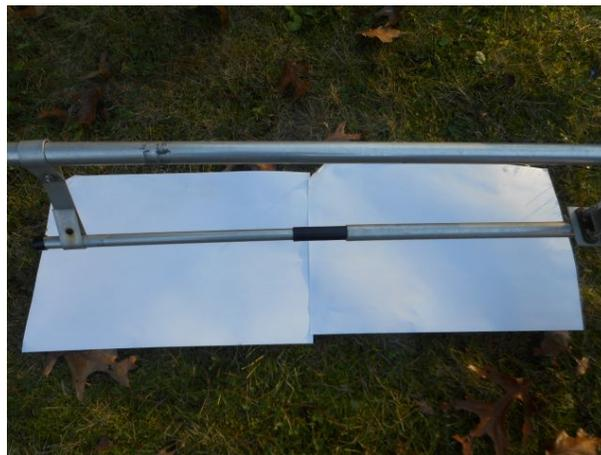
Figure 2. Gamma Match (Boom is just off the right edge of the picture).
