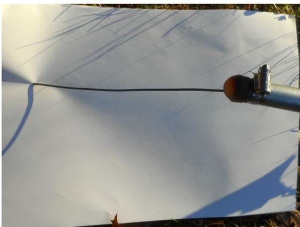
Figure 1. Wire Extension to Yagi Element.
